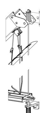
Using sloped blinds it is necessary to achieve correct wire tension to avoid its big undesirable sag while retracting the blind.
